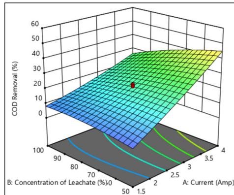
Figure 2. 3D response surface plot of the interaction effect of current and concentration of leachate on COD removal
