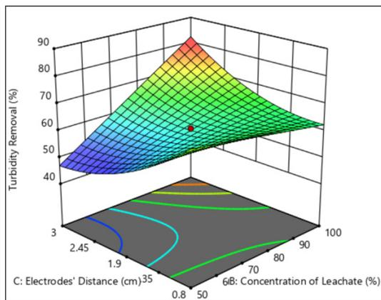
Figure 6. 3D response surface plot of the interaction effect of concentration of leachate and electrodes' distance on turbidity removal
