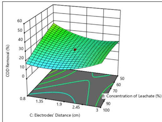
Figure 4. 3D response surface plot of the interaction effect of leachate's concentration and electrodes' distance on COD removal
