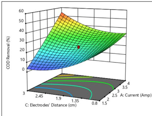
Figure 3. 3D response surface plot of the interaction effect of current and electrodes' distance on COD removal
