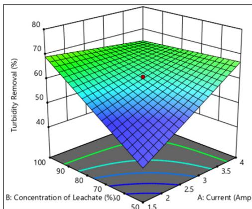
Figure 5. 3D response surface plot of the interaction effect of current and concentration of leachate on turbidity removal
